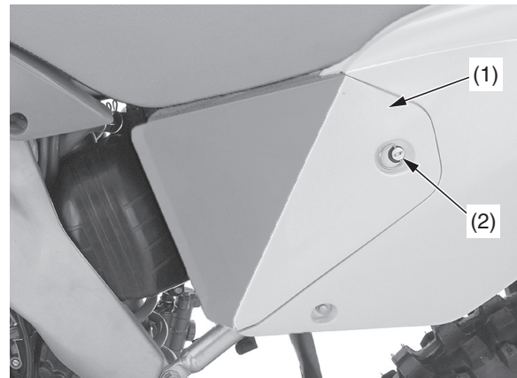
(1) air cleaner housing cover (2) quick fastener
