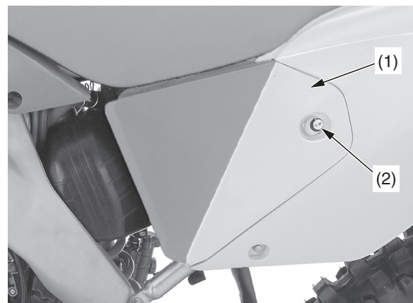
(1) air cleaner housing cover (2) quick fastener
