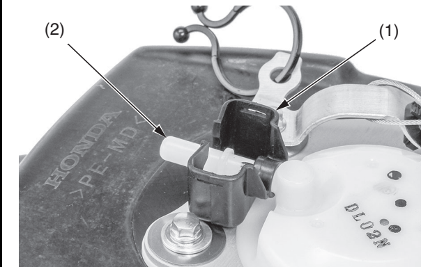
(1) rubber cover (2) fuel joint
