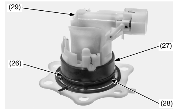
(26) O-ring (new) (27) collar A (28) collar B (29) fuel pump unit
