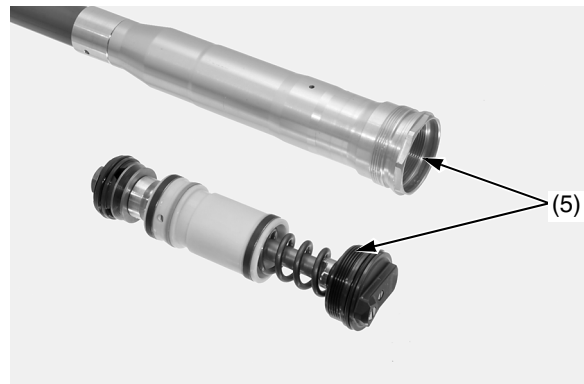
(5) fork bolt and fork damper assembly threads
