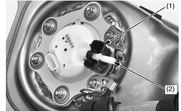
(1) rubber cover (2) fuel joint
